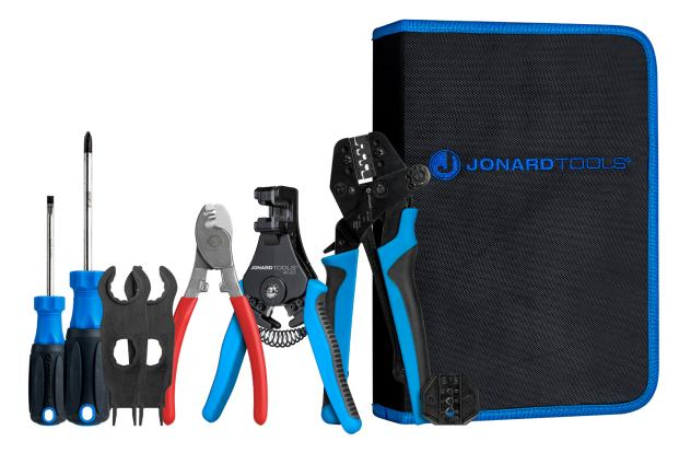
This tool kit is designed to facilitate the installation and maintenance of solar panels. It includes a crimper with MC3 and MC4 dies to crimp connectors onto 14, 12 or 10 AWG (2.5/4.0) (6.0mm2) solar panel wire, solar panel spanners for locking/unlocking connectors, and many other tools.
