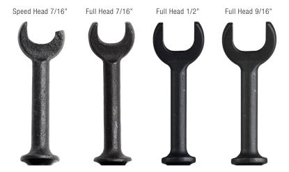
Designed for F Connectors, these torque wrenches provide a perfectly calibrated amount of torque to prevent damage from over-tightening or signal loss from under-tightening. The TWAF wrenches have full-size open heads while the TWAS wrenches have speed heads to skip over the corners of nuts and bolts so no repositioning is required. All Jonard torque wrenches feature:
