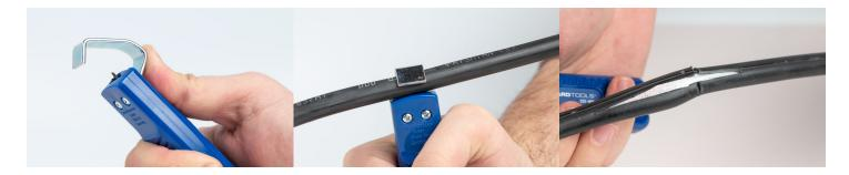
Designed for the fast and precise removal of round cable jackets 8 to 28 mm in diameter. This round cable stripper features the following:
