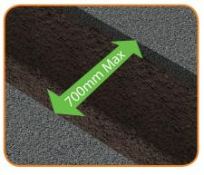
**1.** Ensure max trench width less than 700mm. Assess trench stability prior to install.
