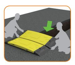
**7.** Lower next plate at an angle so the connectors fit into the slots.
