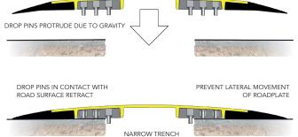
**INTEGRAL DROP PINS INCREASE** PRODUCT STABILITY. ALWAYS CHECK THE DROP PINS ARE IN GOOD WORKING ORDER.
