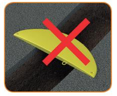
**12.** End section is not load bearing. Do not place end section over trench.
