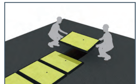
Repeat until the entire trench is covered.
