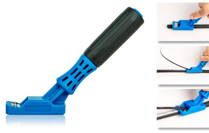
Designed to shave a longitudinal access window in round FTTH riser cables and microducts for mid-span access. This riser slitting tool is perfect for making access windows on cables 8 to 14 mm (0.33" to 0.55") in diameter without damaging the fiber inside. This tool features the following:
