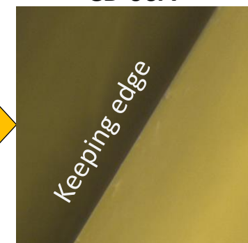
Blade edge after cleaving 250um fiber 10000 times
