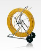
2in1 concept: cable pulling device with detection function Polykat® fibreglass profile Ø 11 mm with integrated copper wires fitted with rod end with external M12 and screwed-on guide head Ø 18 mm connection box for connecting transmitter (1 connection) galvanized steel frame with reel Ø 1000 mm, portable roller supported rod guidance
