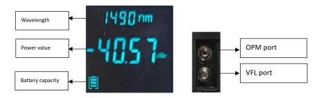
**4.** You can also change the display results from dBm to dB using the dB/dBm key.
