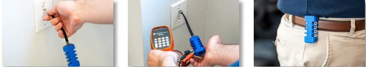
The Jonard Tools BAN-800 8P Modular Adapter, also known as an 8P Banjo, is perfect for connecting butt sets, telephone test sets, tone generators and network test equipment to data and telephone lines using modular plug connections in order to test the data and signals being carried. This 8P Modular Adapter also features the following:
