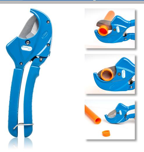
Designed to cut large fiber ducts up to 64 mm (2.52") in diameter, this fiber duct cutter is perfect for cutting PVC, CPVC, PE, HDPE, PEX and other nonmetallic tubing. This fiber duct cutter features the following:
