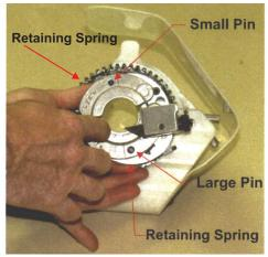
STEP # 4. Choose the bushing with the number that matches the cable gage indicating the cable size in the previous step. Insert the bushing into the tool head by pushing the retaining spring in and sliding the bushing into the bushing holder. The bushings will only go in one way because they have different diameter holes that fit on different size pins.
