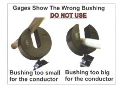
STEP # 3. Determine the bushing needed by using the cable gage and a grip all stick (shotgun). Push the gage on the cable. The cable should go half way down the gage as shown above. If the cable will not go into the gage, the bushing is undersized and should not be used. If the cable drops fully into the gage, the bushing is oversized and should not be used.
