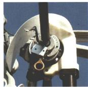
STEP # 8. Using the shotgun, move the MTS Tool Stop to the left of the tool head the distance that you want the strip length to be. Put slight pressure against the tool in the direction of the clamp and begin turning the handle clockwise until the blade begins to strip the insulation.
