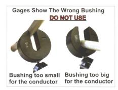
STEP # 3. Determine the bushing needed by using the cable gage and a grip all stick (shotgun). Push the gage on the cable. The cable should go half way down the gage as shown above. If the cable will not go into the gage, the bushing is undersized and should not be used. If the cable drops fully into the gage, the bushing is oversized and should not be used.
