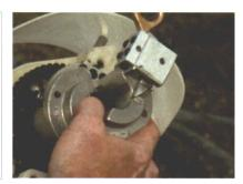
STEP # 4. Choose the bushing with the number that matches the cable gage number that indicated the cable size in the previous step. Insert the bushing into the tool head by pushing the retaining spring in and sliding the bushing into the bushing holder. The bushings will only go in one way because they have different diameter holes that fit on different size pins. Slide the bushing half without the blade into the tool first. Then repeat the operation for the bushing half with the blade.
