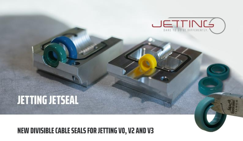
We have recently upgraded our cable seals for Jetting VO (16 mm), V2 and V3 to a new design based on the high-performance material: Material TPU 90Sha. With a hardness of 90 Shore, this material provides an optimal balance of flexibility and durability. TPU (thermoplastic polyurethane) is a rubber-like plastic material that brings several advantages to enhance seal performance and lifespan:
