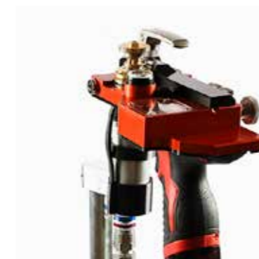
TriggAIR close up with focus on 5/7 ducts
