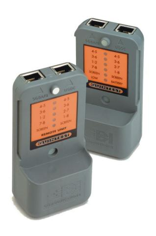
Low Cost Structured Cabling "Wire Map" Tester
