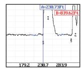
Simple, clean trace interface provides necessary information for fast assessment of fiber run.
