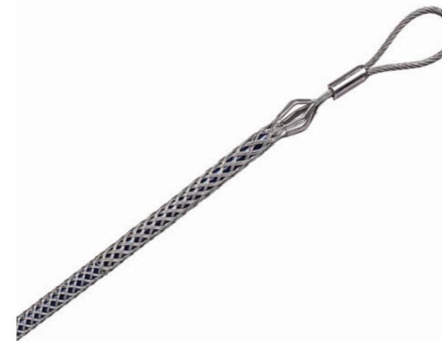
Picture 3 - Cable grip for overhead cabling (Aluminium ferrule at start of mesh, galvanized steel strand, triple back weave)
