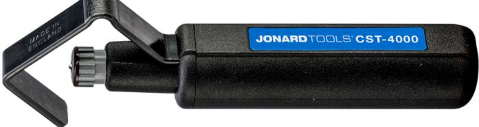
The **PATENTED** CST-1900 and CST-4000 Round Cable Strip & Ring Tools are designed for fast and precise removal of cable jackets from round cables. The CST-1900 removes cable jackets 3/16" to 1 1/8" (4.5 mm to 29 mm) in diameter and the CST-4000 removes cable jackets 3/4" to 1 5/8" (19 mm to 40 mm) in diameter. These round cable strippers feature the following:
