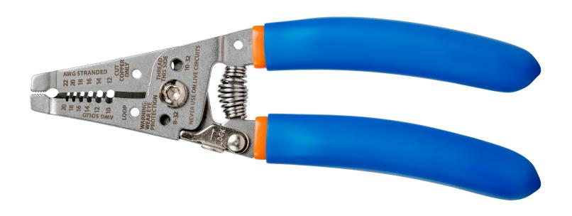
Designed to cut and strip the most commonly used stranded and single conductors, this wire stripper is the perfect tool for cutting and stripping solid wires from 10 to 20 AWG (2.60 to 0.81 mm) and stranded wires from 12 to 22 AWG (2.05 to 0.65 mm). This wire stripper features the following:
