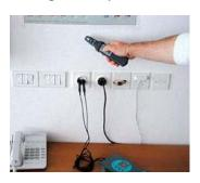
With various arrangements a detection depth between 40 and up to 200 cm can be reached on energized lines, a detection depth up to  $40\,\mathrm{cm}$  can be reached on non-energized lines.
