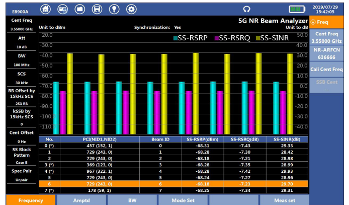
Figure 6: 5G NR beam analyzer measures up to 8 beams at once..
